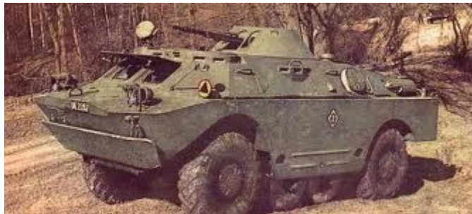
BRDM-2 Armoured Recce Vehicle (note the 2xMagnesium alloy auxiliary wheels lowered)
